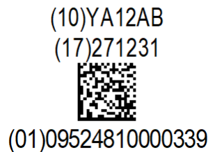
Figure 4.14-3. Example of split HRI placement
