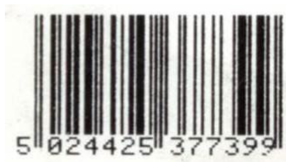
Figure 5.12.5.12-1. Symbol with edge determination problem
