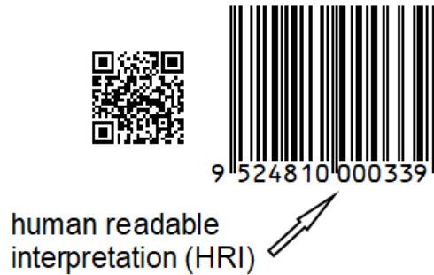
Figure 4.14-7. Example of adjacent barcode HRI
