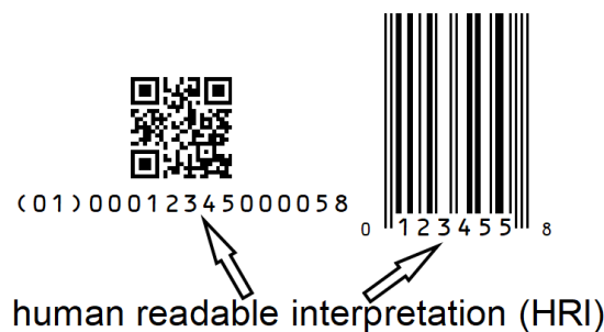
Figure 4.14-9. Example of adjacent UPC-E barcode HRI
