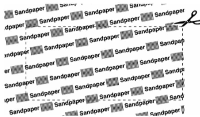
Figure 6.3.3.7-2. Barcode placement on random-wrapped item
