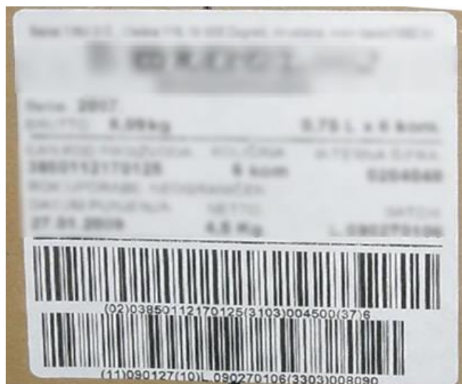
Figure 7-6 Example of incorrect use of AI (02) and (37) (there is no AI (00) SSCC)
